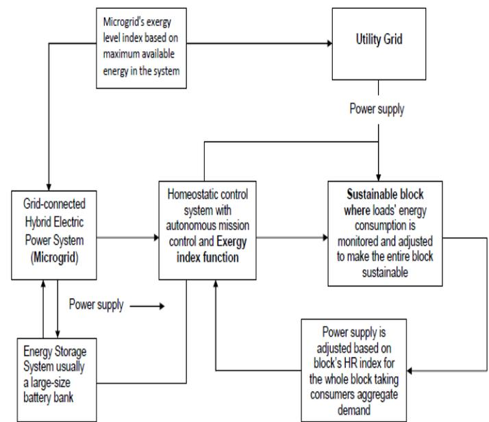
**Fig.1.** A particular example of the homeostatic control (HC) model for SHES. Here both energy and exergy management are built in the SHES to enable resilience and sustainability [10,18,19,21,22]. Source: owned elaboration
