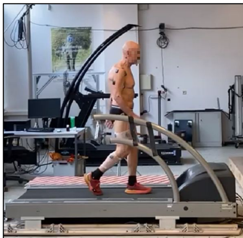
Fig. 1.1 Participant equipped with 21 retro-reflective markers and 16 wireless EMG sensors on the right side, during treadmill walking.
