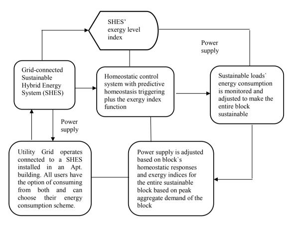
Fig. 1. The diagram illustrates how homeostatic control mechanisms based on reactive and predictive homeostasis trigger a system's sustainability stress response that imposes a restraint over energy consumption of loads based on the energy supply being available in the SHES. Source: Own elaboration.
