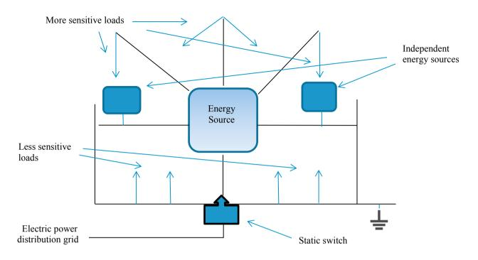
Fig. 3. A diagram representing a HC model which illustrates an example of a potential microgrid architecture with several energy sources and loads. Source: adaptation of Fig. 1 in "Microgrid concept (Electrical point of view)" [20].
