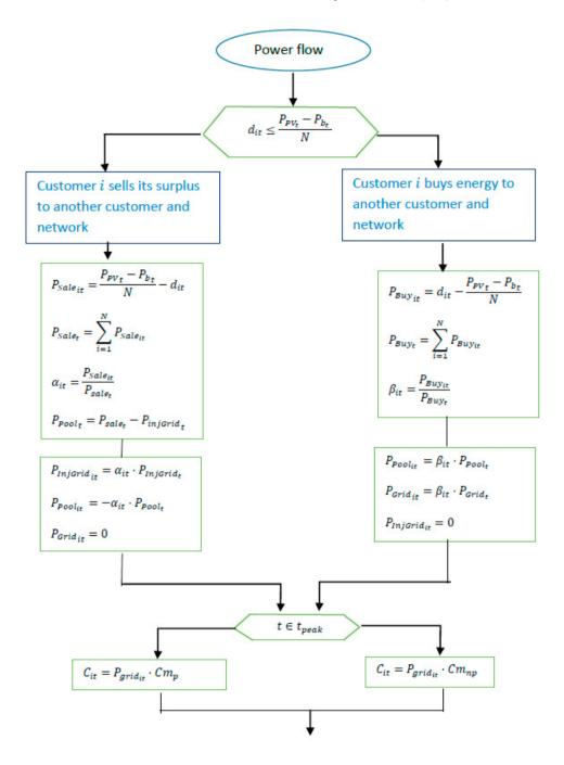
Fig. 2. Above it is shown a particular criterion based on (homeostatic control) HC which permits the energy exchange between the utility's customers and the electric power distribution grid. Source: Own elaboration.
